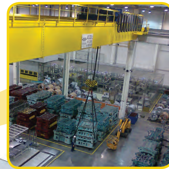
STAMPING DIES MANAGING CRANES 冲压模具用起重机
