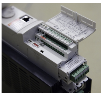
12 / Hoist Frequency inverter
